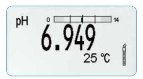
The CMC function (Continuous Measurement Control) of a pH 3310 informs you whether you are measuring inside the calibrated range. An alert is given as soon as you are outside the limits.
